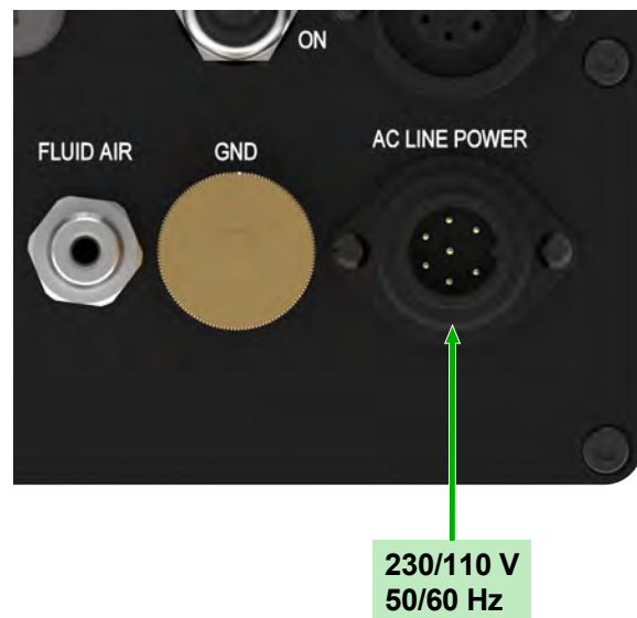
Illustration 4: Connection for the power cable on the rear of the control module
